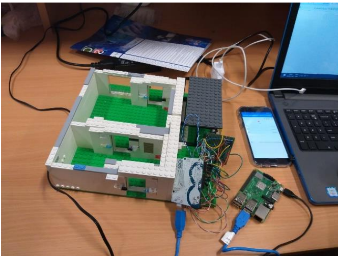
This was our first try: sensors integrated in a LEGO model
